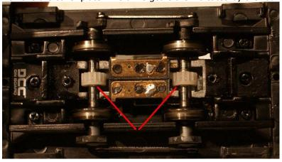
Remove the wheel set. Clean the wheel contact wipers if they are dirty. Note the gears inside the engine.
