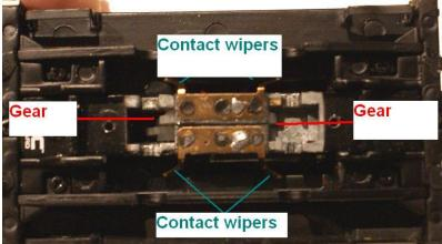
With the DCC logo to your left as shown, install the new wheel set so that the solid sides of the gears are
