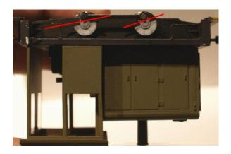
When you apply the cover plate, the pressure on the wheels may quarter them. If not, remove the side rod pins one at a time and enlarge the holes in the side rods (see red arrows) to allow more flexibility.
