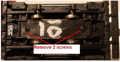
Remove the cover plate. The drive gears are indicated by the red lines.
